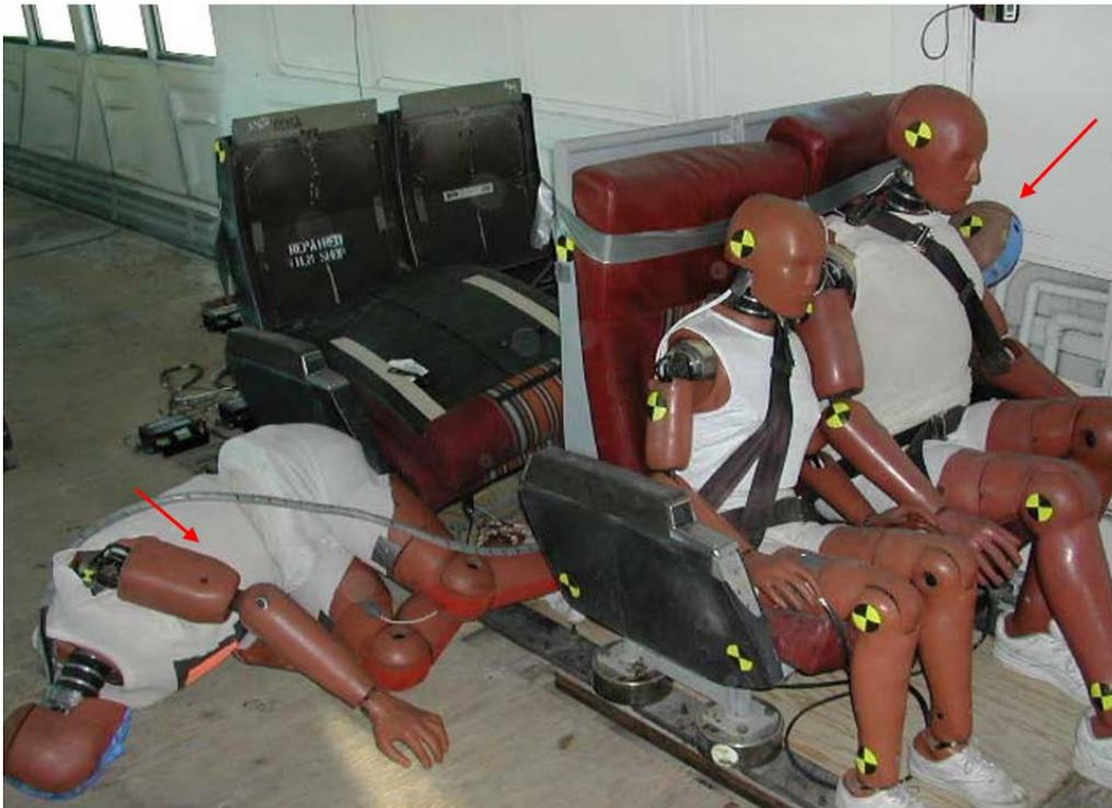
Figure 4. Post-test front angled view of landing positions of two unrestrained crash dummies (see red arrows) and two restrained crash dummies.<sup>19</sup>
