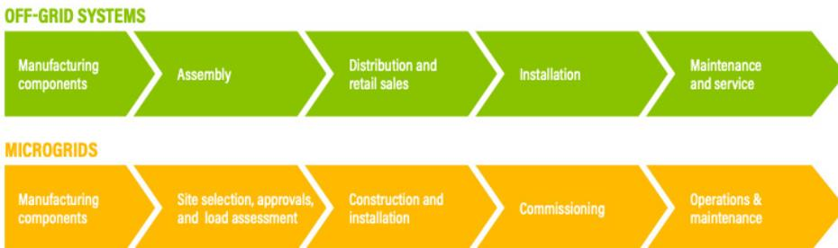
Figure 1: Project lifecycle of off-grid systems and micro-grids. Adapted from IRENA, 2012<sup>4</sup>
